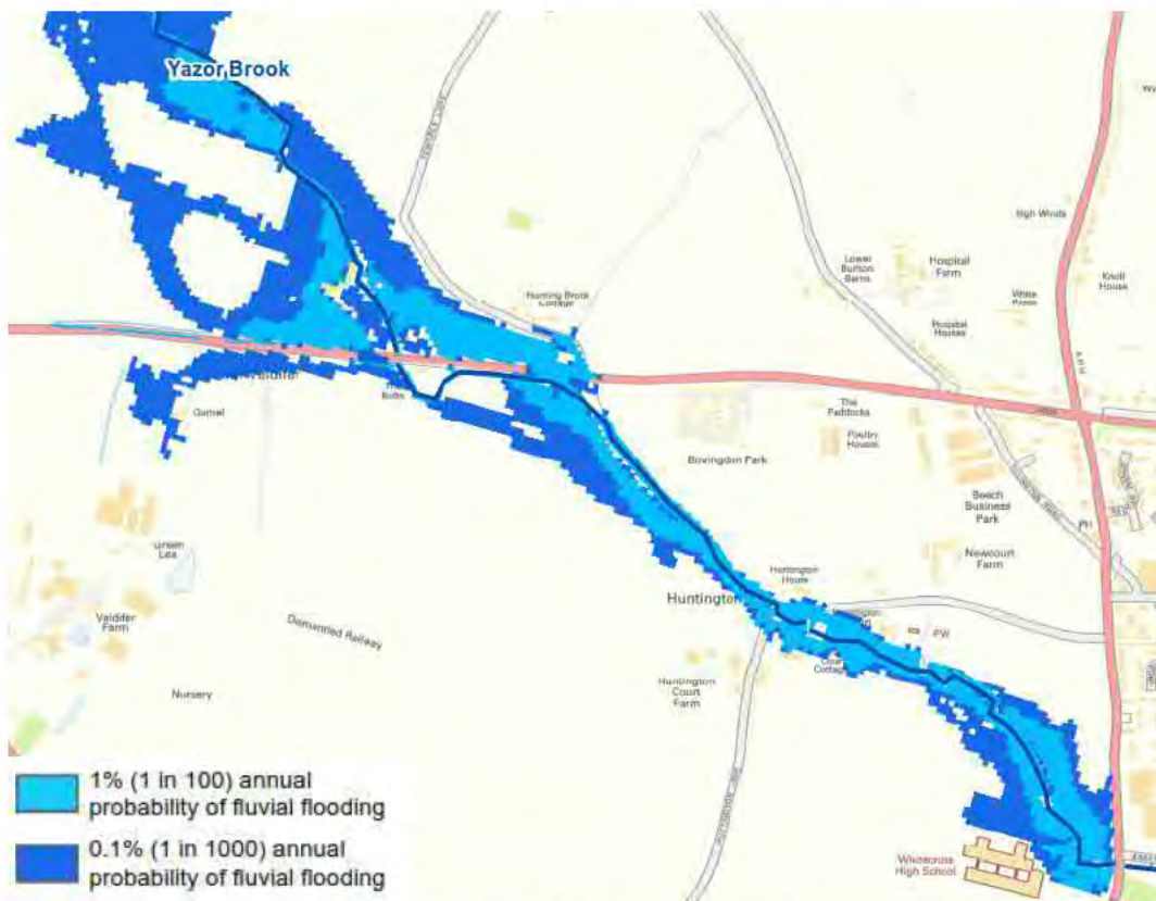
Figure 10-20: Yazor Brook hydraulic modelling with FAS
