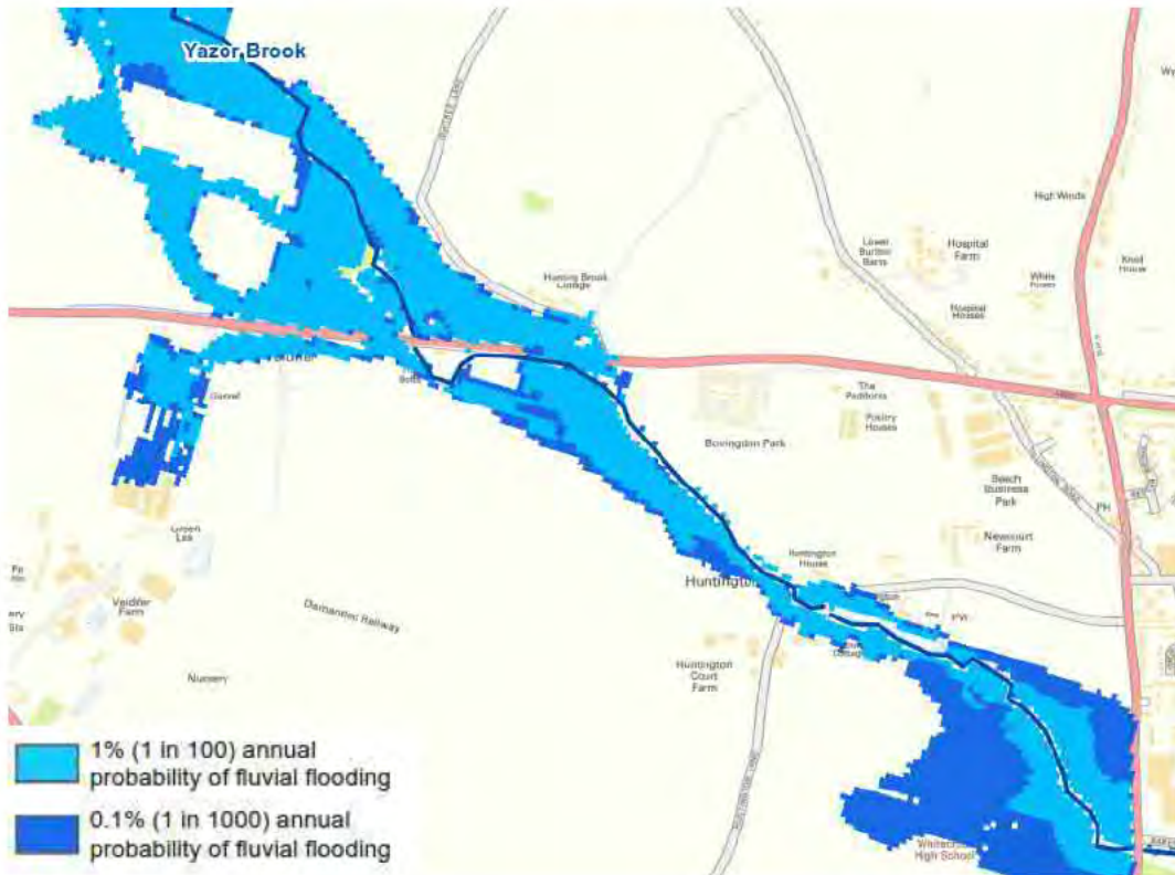
Figure 10-19: Yazor Brook hydraulic modelling without FAS
